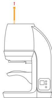
5. Remove the M5x100mm bolt.
