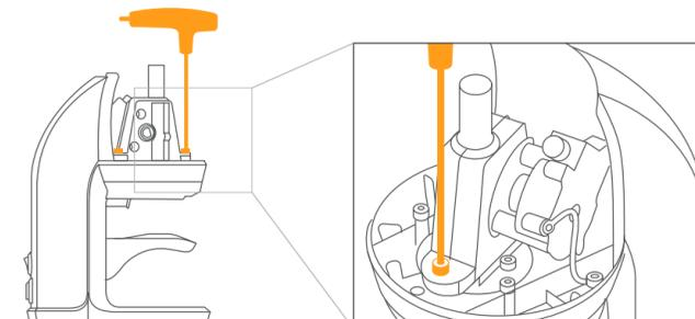
13. Remove both M5 bolts from the motor frame with the Allen key.
