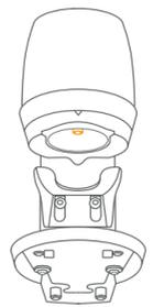
9. Check if the tamper shaft is in the lowered position.
