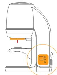
1. Put the unit in CLEAN mode by pressing the CLEAN button.
