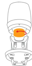
11. Insert the tamper base. (NOTE: left-handed thread)
