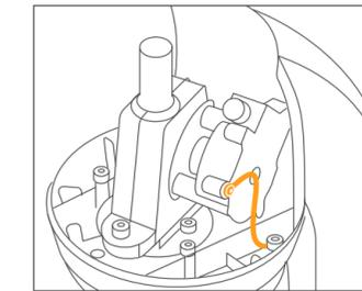
12. Remove the earthing cable from the motor.
