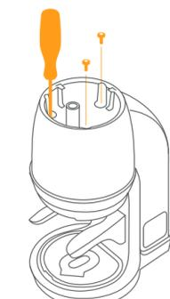
10. Remove three M4 bolts with the yellow screw driver.
