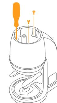
6. Fasten the middle cover with 3 screws using the yellow screw driver.
