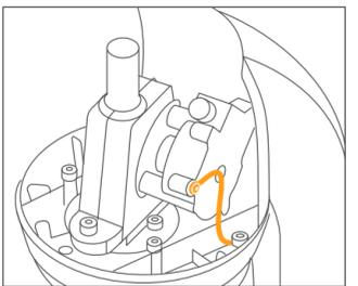
4. Connect the earthing cable to the motor.
