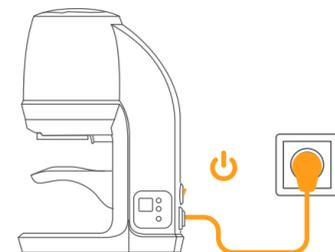
7. Insert the Power Cable, switch ON the unit and activate the CLEAN mode.
