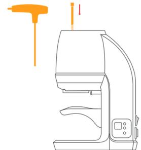
12. Fix the tamper base with the M5 bolt using the Allen key.
