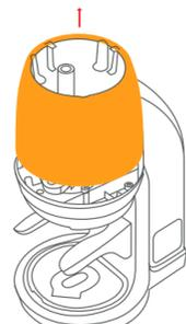
5. Install the middle cover and make sure it is neatly aligned with the main body.
