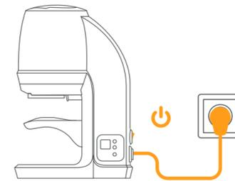
14. Insert the power cable and switch ON the unit.
