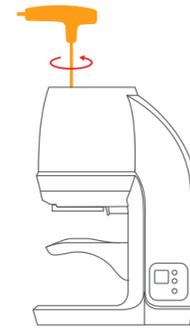
4. Unscrew the M5x100mm bolt with the Allen key.
