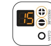
In **standby mode**, press and hold '+' and '-' button for **3 sec.**
