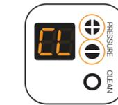
1. Press the 'CLEAN' button to bring tamper in cleaning position. Now press and hold '+' and '-' button for **3 sec.**
